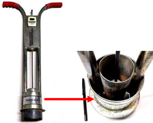
Fig.2 The double ring infiltro-meter Turf Tec
