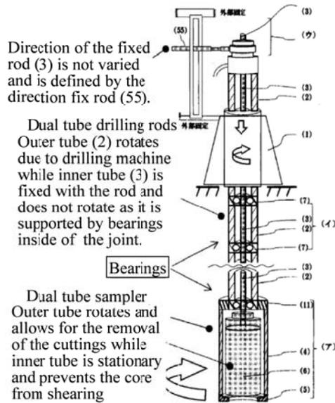
Fig. 5 Drilling/sampling systems used for oriented core samples
