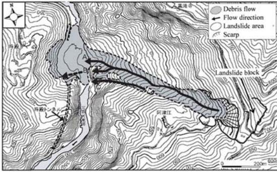
(a) Plan view of the site of slope failure and debris flow in the landslide area [14]
