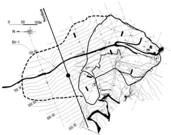
(b) Plan view of the landslide block
