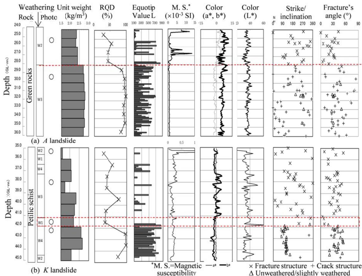
Fig. 10 Results of measurement and image analysis of core samples from the A and K landslides
