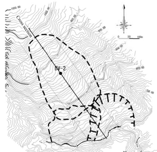
(a) Plan view of the landslide area
