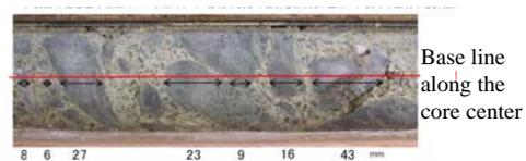
Fig. 6 Base line marked on the borehole core
