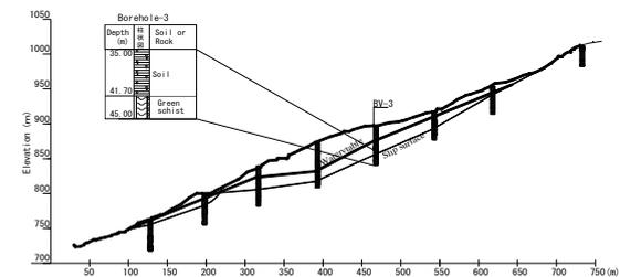
(b) Cross section of the landslide block
