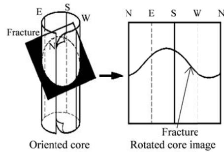
(a) Oriented 360° core and rotated core image
