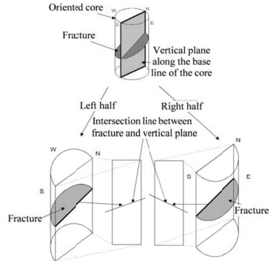
(b) Calculation of strike and dip of planar fracture
