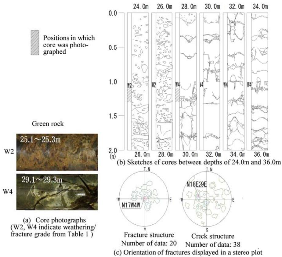
Fig. 8 Observation of core samples from the A landslide
