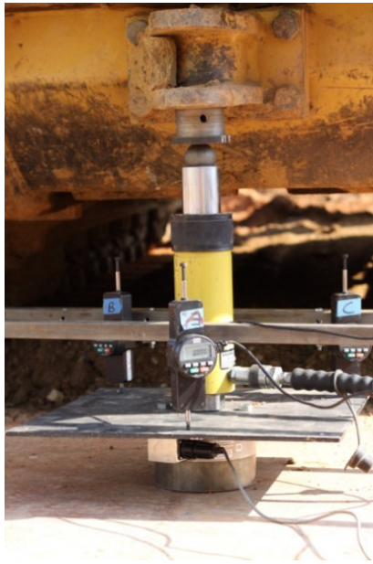
Fig. 10: Photo showing plate load test setup
