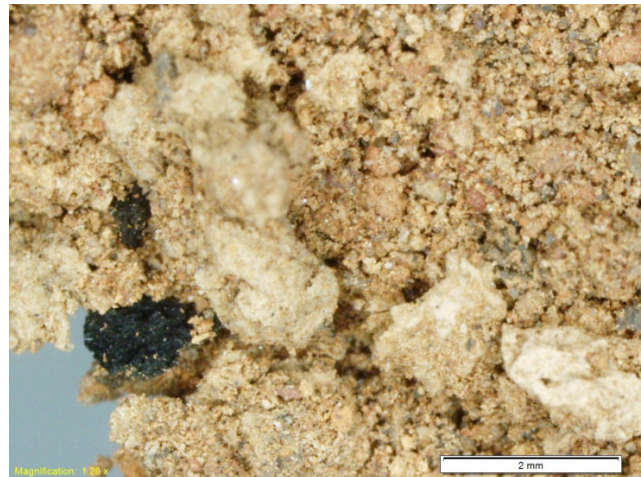
Fig. 1: Stereomicroscope image of the DA SSA ash
