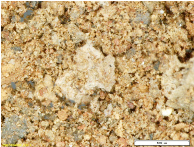
Fig. 2: Stereomicroscope image of SA SSA ash
