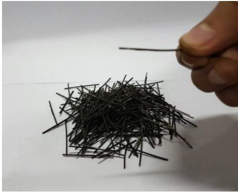
Fig. 4 Steel fibers in 1 inch cut length
