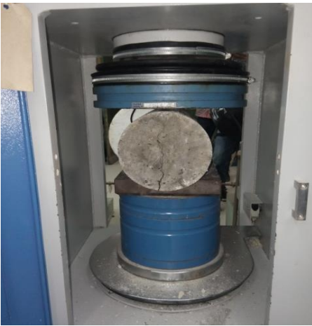
Fig. 7 Splitting tensile test on cylindrical specimens
