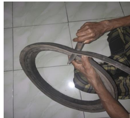
Fig. 2 Cutting process of waste tyre to obtain extracted steel fibers
