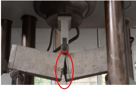
Fig. 12 Crack opening in POFA concrete with SFEFWT
