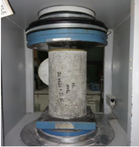
Fig. 6 Compressive test on cylindrical specimens
