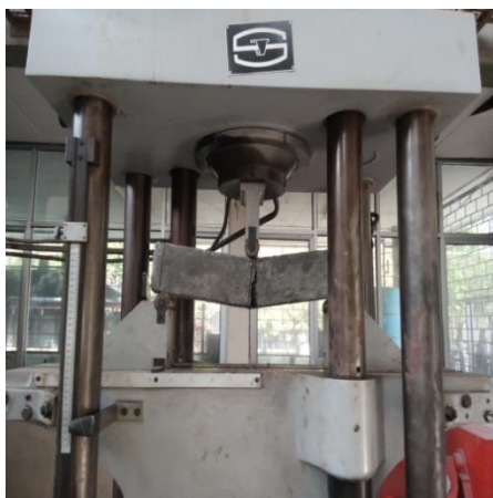
Fig. 8 Flexural test on beam specimens
