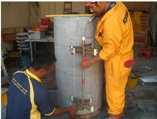
Fig.3(d) Actual Global Strain Extensometer system for spun pile application
