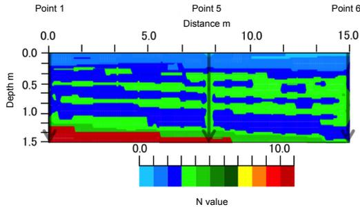
Fig. 9 Distribution by Kriging on Point 1, 5 and 6 with 0.25m pitch
