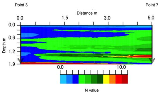
Fig. 11 Distribution by Kriging on other cross section
