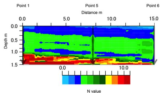
Fig. 8 Distribution by Kriging on Point 1, 5 and 6 with 0.01m pitch
