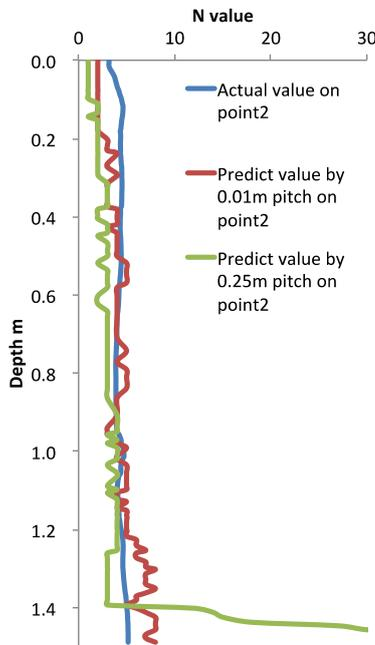
Fig. 10 Comparison between measured and predicted values with 0.01 and 0.25m pitch
