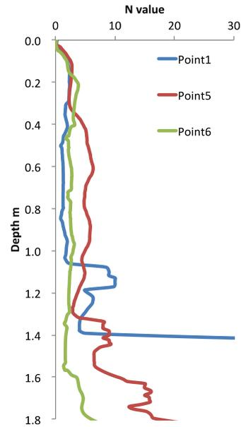
Fig. 6 Measured values on Points 1, 5 and 6
