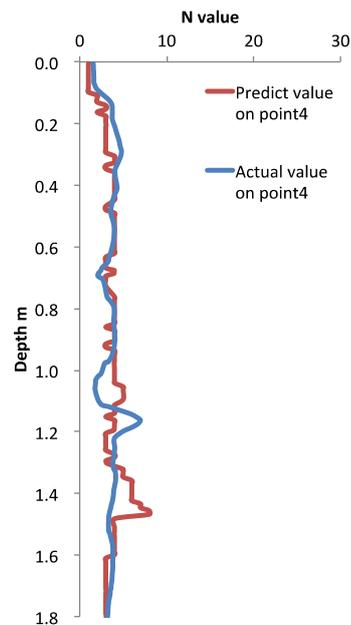
Fig. 13 Comparison between measured and predicted values on point 4
