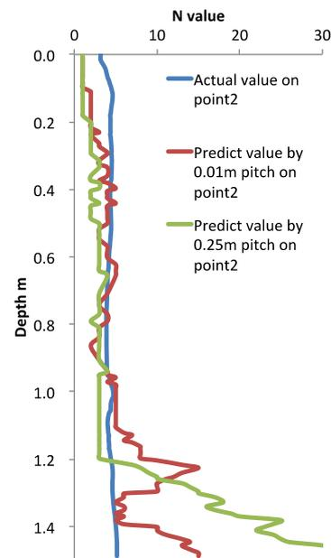
Fig. 7 Comparison between measured and predicted values on point 2 with 0.01m pitch
