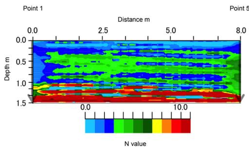
Fig. 4 Prediction by Kriging with 0.01m pitch
