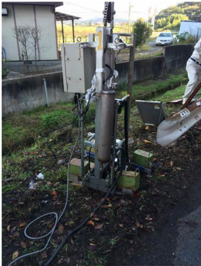
Fig. 1 New-typed Swedish sounding testing machine (NSWS)
