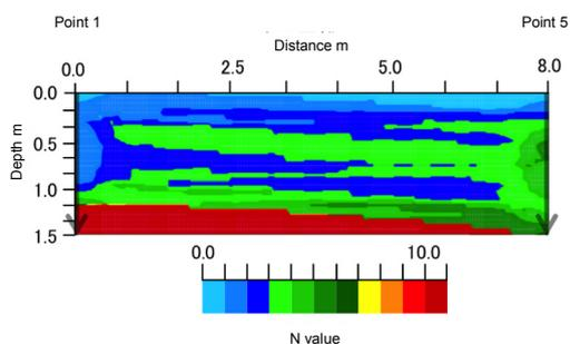
Fig. 5 Prediction by Kriging with 0.25m pitch
