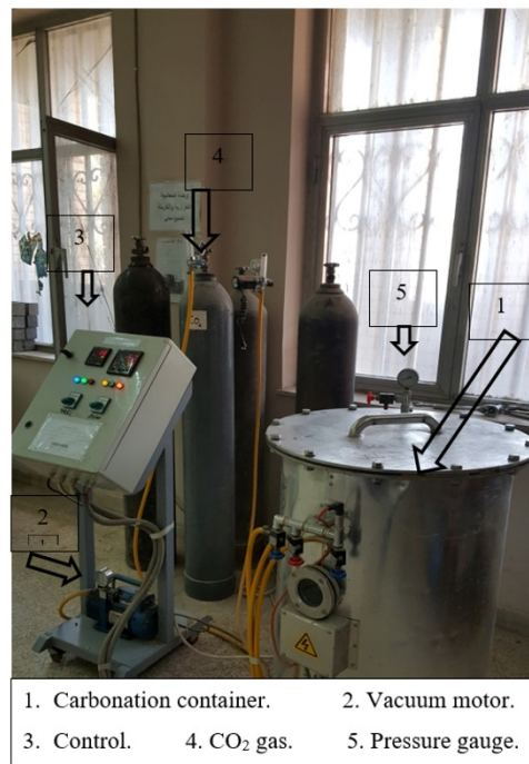
Fig.2 Carbonation apparatus.
