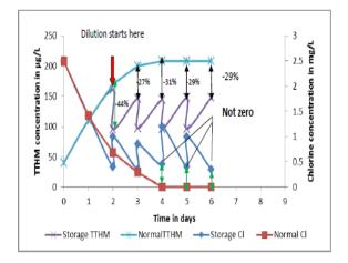
Fig. 2 Storage Tank run vs. Normal run chlorine residual and TTHM trends. The percent differences between the TTHM formation and chlorine decay values are also noted.
