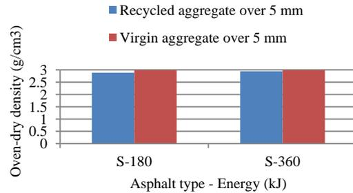
Fig.14 Oven-dry density of recycled aggregate over 5 mm from straight asphalt specimens
