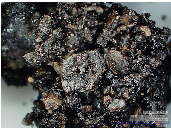
Fig.9 Residues under 2.5 mm containing extracted asphalt binder
