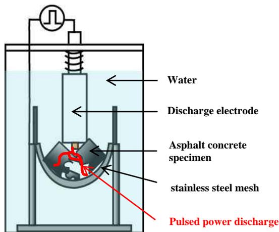
a) Pulsed power discharge into specimens on 5 mm apertures stainless steel mesh
