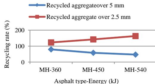
Fig.11 Recycling rates of modified type- H asphalt concrete aggregate
