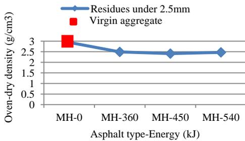
Fig.17 Oven-dry density of residues from modified type-H asphalt specimens and virgin aggregate under 2.5 mm
