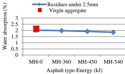
Fig.21 Water absorption of residues from modified type-H asphalt specimens and virgin aggregate under 2.5 mm
