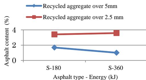
Fig.12 Asphalt content of recycled aggregate from straight asphalt concrete specimens
