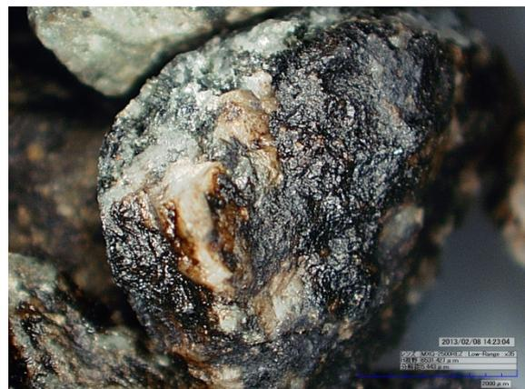
Fig.7 Partially-coated piece of aggregate
