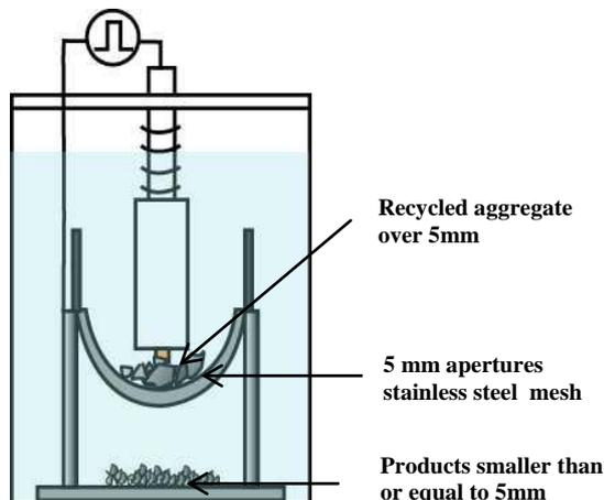
b) Production of recycled aggregate over 5 mm
