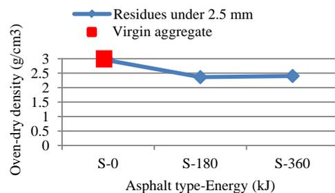
Fig.16 Oven-dry density of residues from straight asphalt specimens and virgin aggregate
