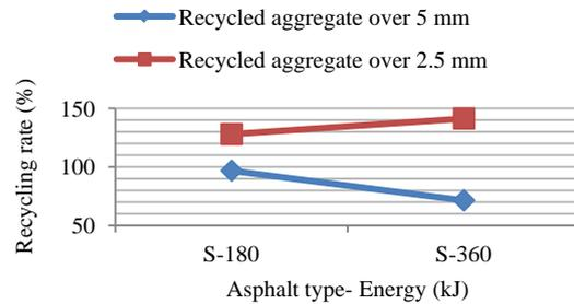
Fig.10 Recycling rates of straight asphalt concrete aggregate
