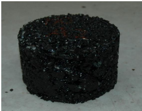
Fig.1 Asphalt concrete specimen
