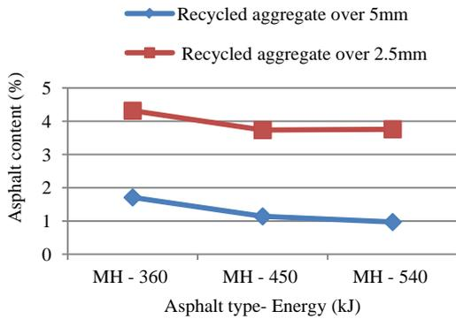
Fig.13 Asphalt content of recycled aggregate from modified asphalt concrete specimens
