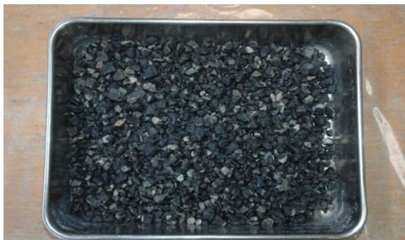
Fig.4 Recycled aggregate larger than 2.5 mm
