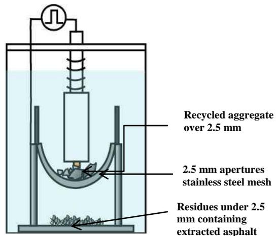
c) Production of recycled aggregate over 2.5 mm and residues under 2.5 mm
