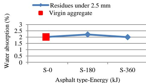
Fig.20 Water absorption of residues from straight asphalt specimens and virgin aggregate under 2.5 mm
