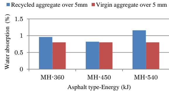
Fig.19 Water absorption of recycled aggregate over 5 mm from modified type-H asphalt specimens and virgin aggregate
