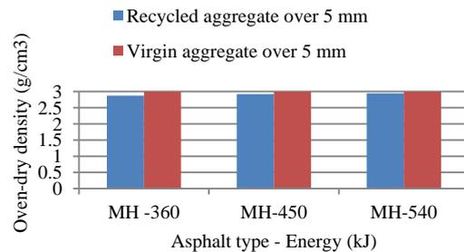
Fig.15 Oven-dry density of recycled aggregate over 5 mm from modified asphalt specimens
