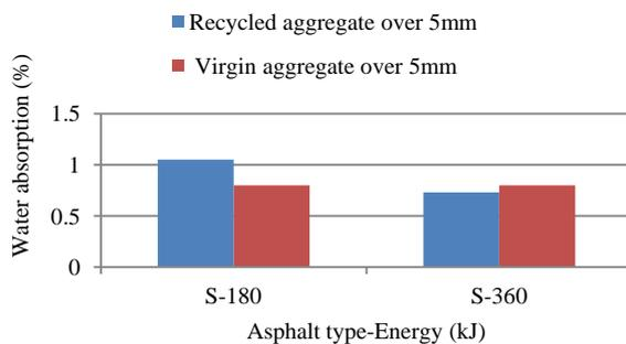
Fig.18 Water absorption of recycled aggregate over 5mm from straight asphalt specimens and virgin aggregate
