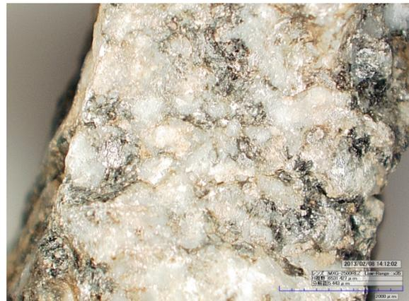
Fig.6 Almost-clean piece of aggregate
