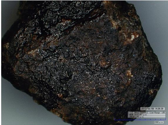
Fig.8 Totally-coated piece of aggregate
