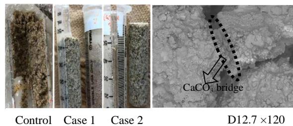
Fig. 10 Status of solidified sand (left images) and SEM images of solidified sand showing the  $\text{CaCO}_3$  bonding in between the sand particles (right images)
