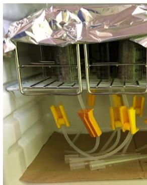
Fig. 3 Status of sand solidification test using extracted crude enzyme
