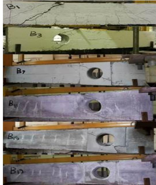
Fig.9. The crack patterns for 150 mm opening.
