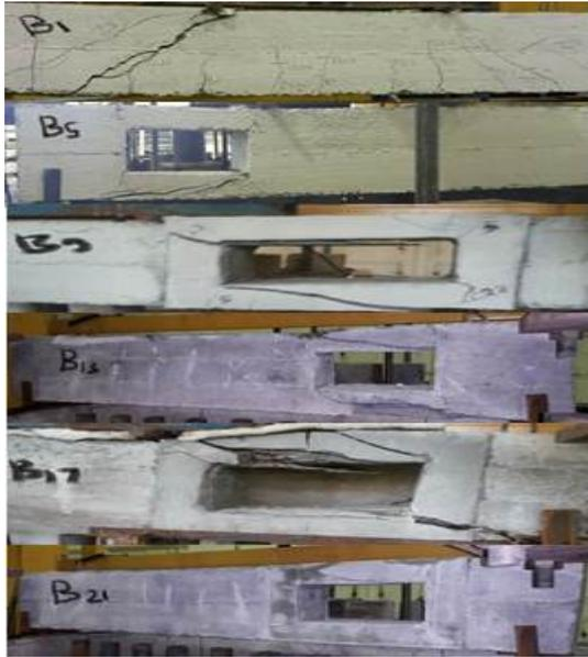
Fig.11. The crack patterns for 150\*300 mm opening.
