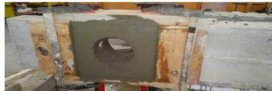
Fig.4. Ferrocement Layer.
