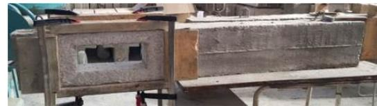
Fig.3. Surface preparation of retrofitted beams.
