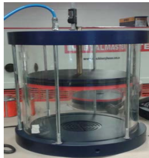
Fig. 1. (a) Schematic diagram, (b) Photo of a pressure chamber used in the experimental program
