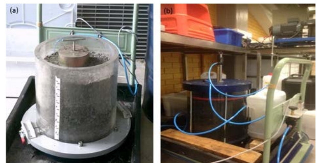
Fig. 3. (a) Compacting spoil into the pressure chamber, (b) Saturation of spoil compacted into the pressure chamber
