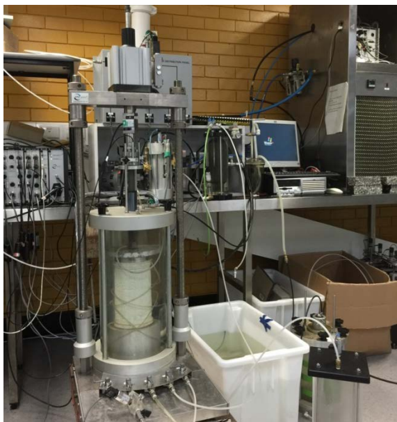
Fig. 5. Triaxial system used for measuring shear strength properties of spoil
