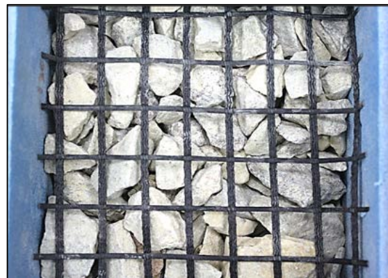
Fig. 4 Geogrid overlying a compacted ballast layer
