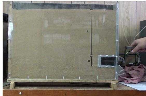
Fig. 2 The tunnel heading model
