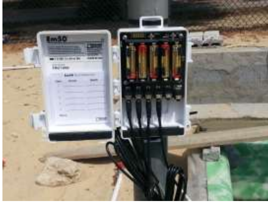
Figure 2. Em50 data loggers used for 5TE sensors
