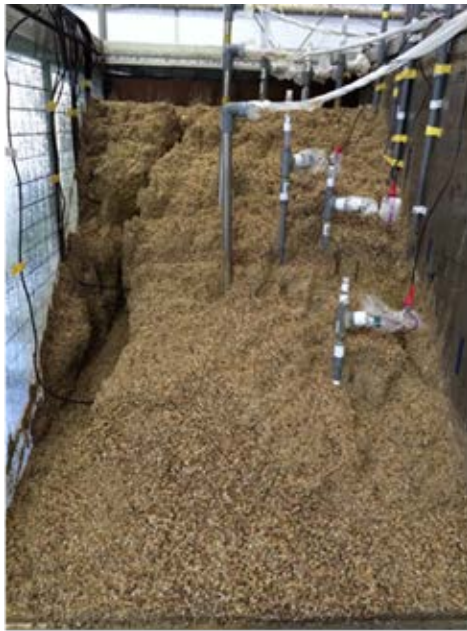
Photo 1 Model slope after experiment (Case 1)
