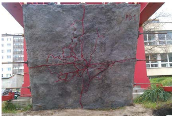
Fig. 14 The course of cracks on the contact surface of experimental post-tensioned slab
