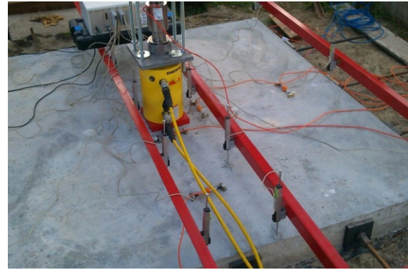
Fig. 7 Potentiometric position sensors for measurement of vertical deformations and built-in pressure sensor for measurement of the vertical load
