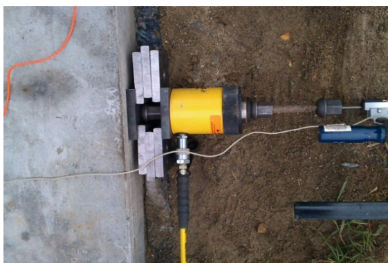
Fig. 3 The prestressing system with hollow hydraulic cylinder
