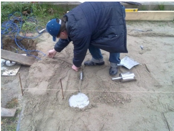
Fig. 5 Installation of geotechnical pressure cells for measurement of the stress on the interface of the slab and subsoil.
