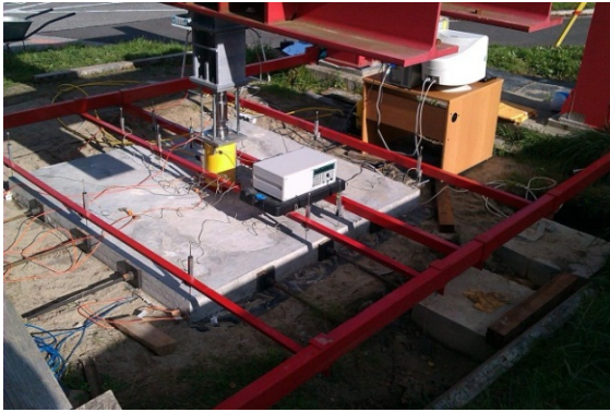
Fig. 4 The prestressing system with hollow hydraulic cylinder
