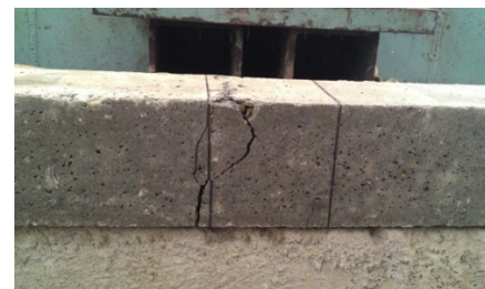
(a). Crack pattern of a beam specimen
