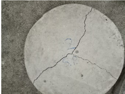
(b). Crack pattern of round panel concrete as tested according to ASTM C-1550-02
