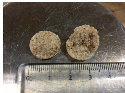
Fig. 10 Solidified parts of sediments using a bacterium obtained from near the Okinawa beachrocks.
