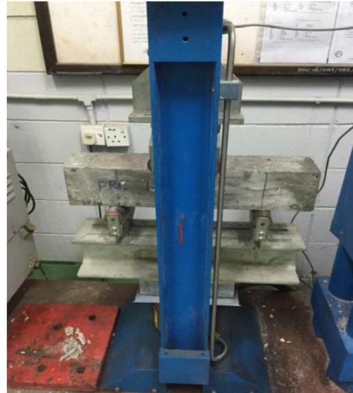
Fig. 9 Determination of flexural strength of concrete
