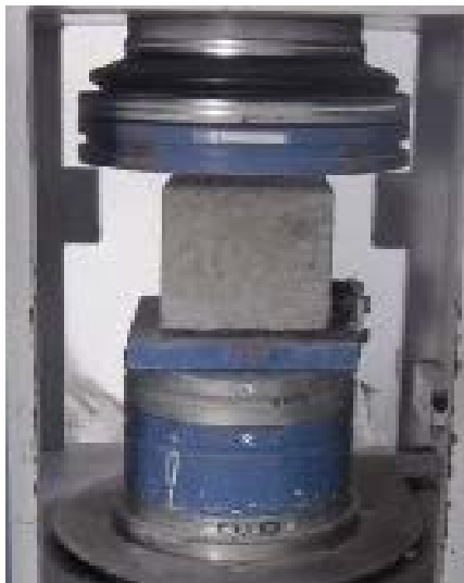
Fig. 3 Testing of concrete cube specimen for compressive strength.
