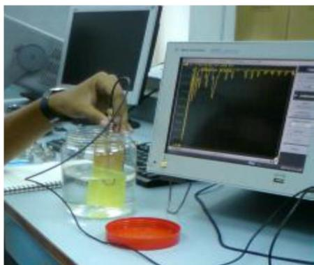
Fig. 2 Reflection measurement for salinity using loop antenna.
