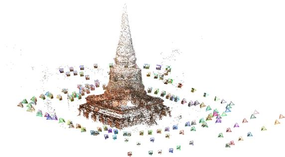
Fig. 8 A 3D model of the temple created from VisualSFM with camera positions.
