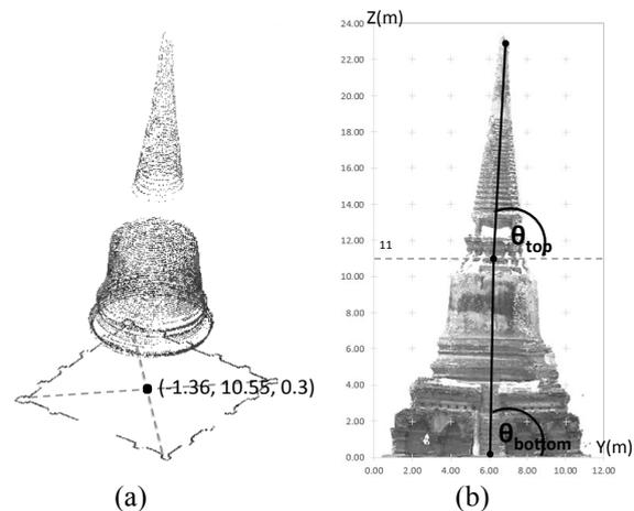
Fig. 10 (a) Show the location of the center of the temple; (b) show angles of inclination of the top and bottom parts of the temple.
