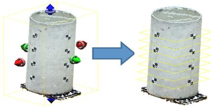
Fig. 6 Examples of horizontal slices used to cut a 3D model.
