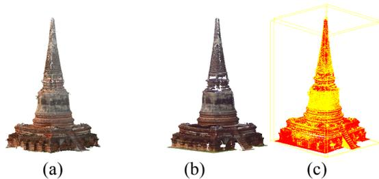
Fig. 9 (a) 3D model from VisualSFM (b) 3D model from LIDAR (c) the results of registration between the model from VisualSFM and LIDAR.
