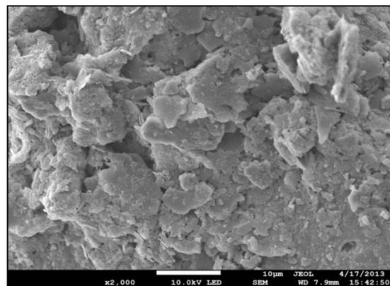
Fig. 6. The morphology photo of optimum soil mixing design by FESEM
