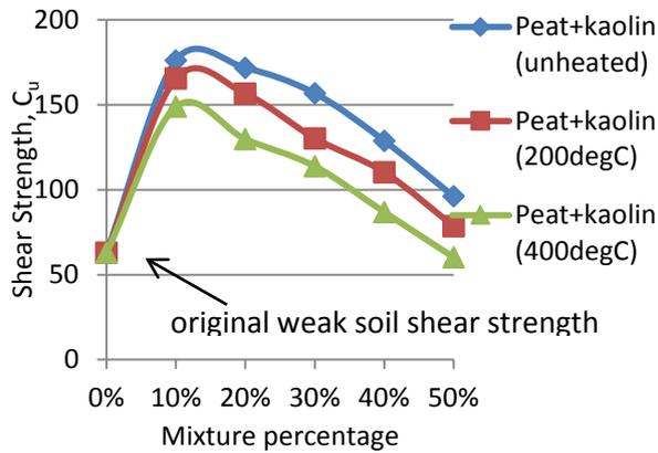
Fig. 2. Graph of shear strength against percentage of soil mixture samples
