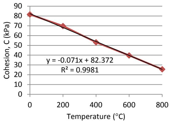
Fig. 3. Graph of cohesion against kaolin temperature of soil mixture samples
