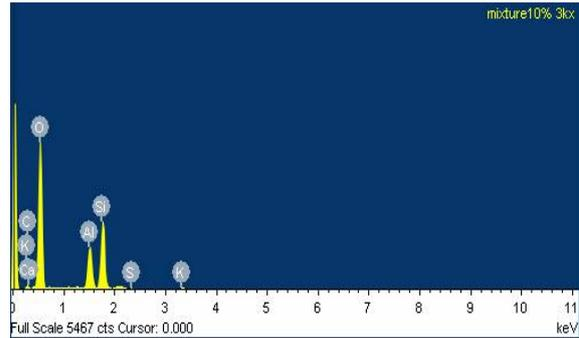
Fig. 5. The EDAX result for optimum design of mixed soil sample
