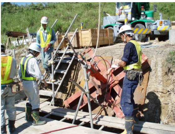
Photo 6 Pullout Test Revealed \tau = 0.5 \text{ MN/m}^2 for a Project in the Makinohara Region
