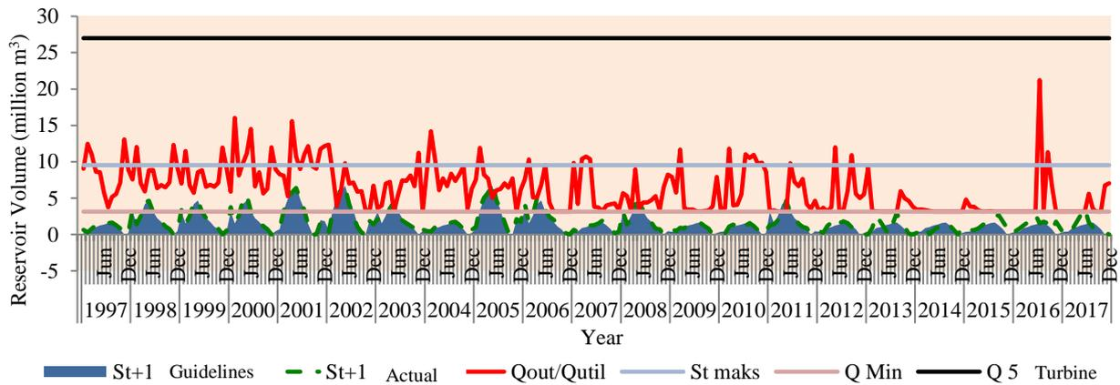
Fig.8 Chart of optimization of the three-class operation pattern of Cileunca Reservoir using the continuous model, 1997–2017
