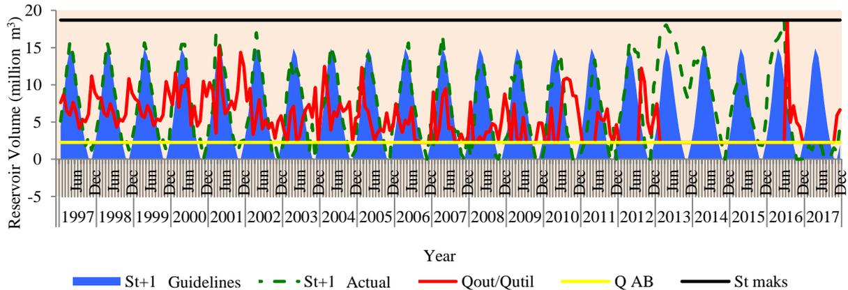
Fig.6 Chart of optimization of three-class operation pattern of Cipanunjang Reservoir using continuous model, 1997–2017
