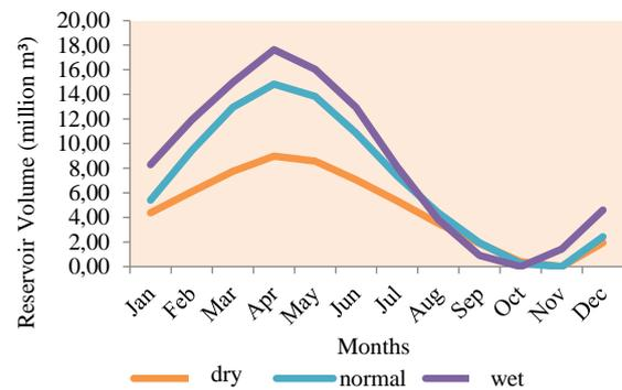
Fig.2 Chart of guidelines trajectory for three-class continuous discharge of Cipanunjang Reservoir
