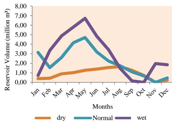
Fig.3 Chart of guidelines trajectory for three-class continuous discharge of Cileunca Reservoir
