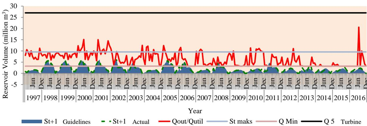
Fig.9 Chart of optimization of the five-class operation pattern of Cileunca Reservoir using the continuous model, 1997–2017
