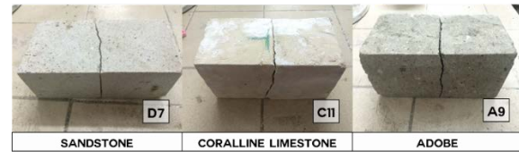
Fig. 4 Failure of masonry blocks due to shear
