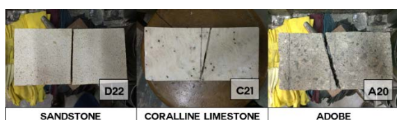
Fig. 7 Failure of masonry blocks due to flexure
