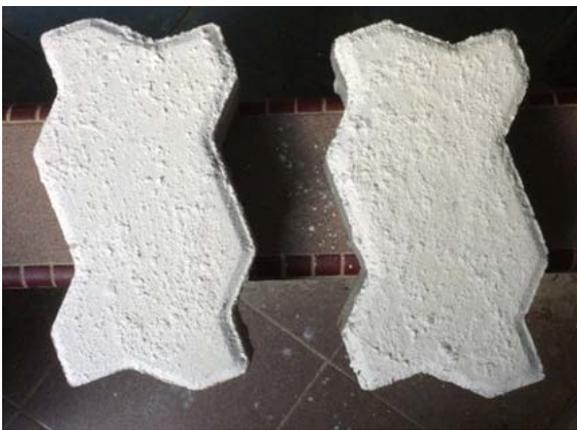
Fig. 4 Concrete pavers coated with coating mixture
