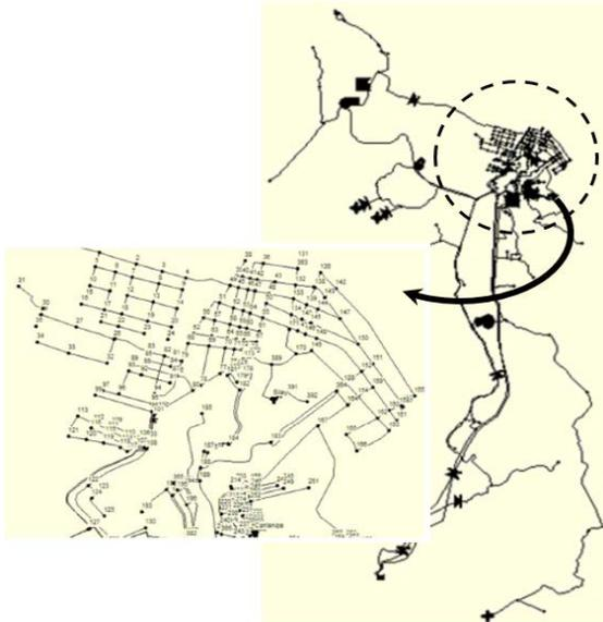
Fig. 1 Water Distribution Network Model
