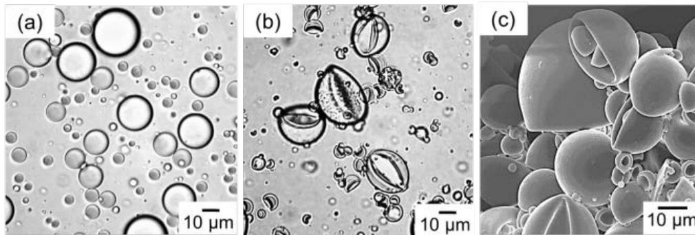
Fig. 4 Optical micrographs of (a) monomer droplets and (b) poly(methyl methacrylate-divinyl benzene)/octadecane microcapsules and scanning electron micrograph of poly(methyl methacrylate-divinyl benzene)/octadecane after washing with 2-propanol
