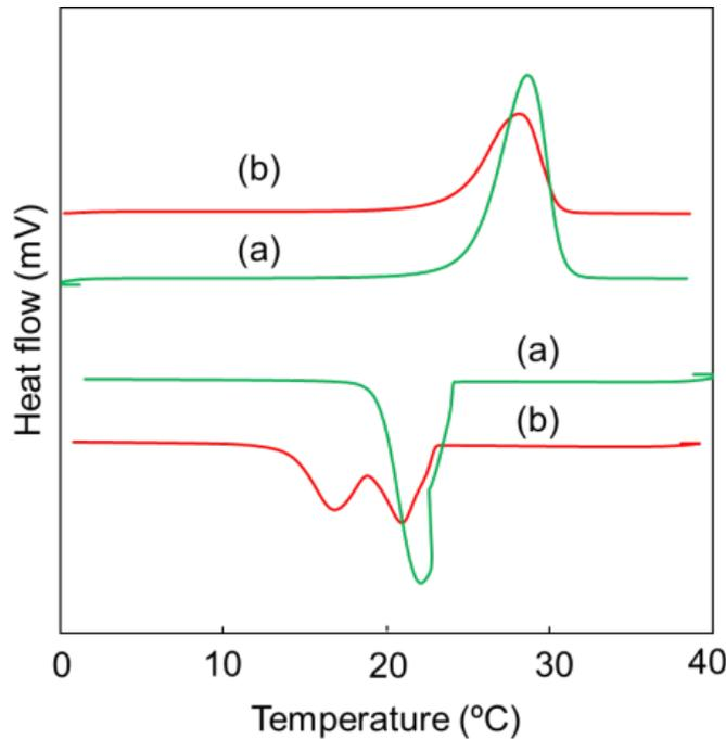
Fig. 6 Differential scanning calorimeter thermograms of bulk octadecane (a) and poly(methyl methacrylate-divinyl benzene)/octadecane microcapsules using methyl methacrylate: divinyl benzene ratio of 90:10 (w/w%) prepared by microsuspension iodine transfer polymerization (b)
