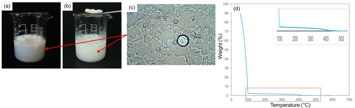
Fig. 2 Suspension photos (a and b), optical micrograph (c) and thermogravimetric thermogram (d) of polymethyl methacrylate/octadecane microcapsules prepared by microsuspension iodine transfer polymerization using various concentrations of chitosan in aqueous medium (wt%): 0.25 (a) and 0.50 (b)
