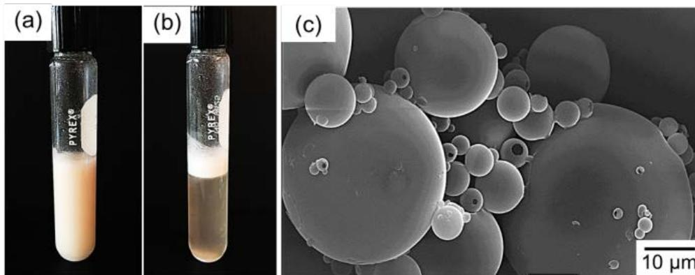
Fig. 3 Suspension photos before (a) and after (b) centrifugation at 3,000 rpm for 15 minutes of polymethyl methacrylate/octadecane microcapsules and scanning electron micrograph (c) polymethyl methacrylate/octadecane microcapsules washed with 2-propanol
