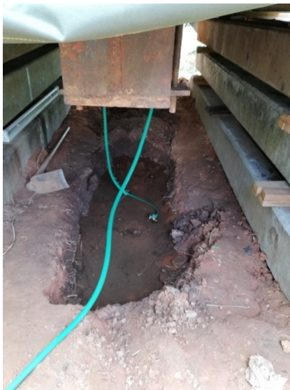
Fig. 15 Wetting pit (soaking for 4 days)
