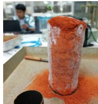
Fig. 10 Specimen after trimming for the testing
