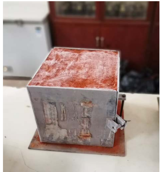
Fig. 4 Frozen undisturbed sample
