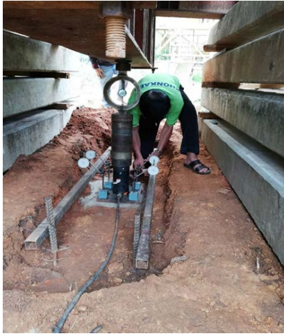
Fig. 14 The installation of the plate bearing test
