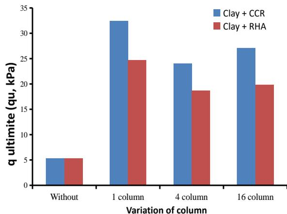
Fig. 11 The value of ultimate bearing capacity for each variation
