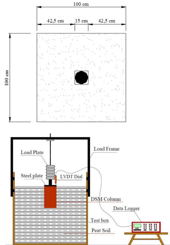
Fig. 5 DSM modeling scheme with 15 cm diameter with 1 column
