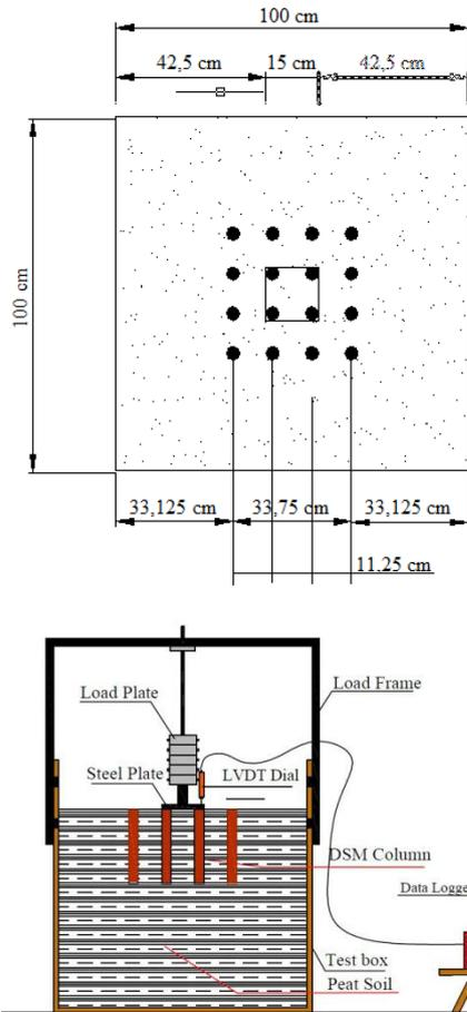
Fig. 7 DSM modeling scheme with 3.75 cm diameter with 16 columns
