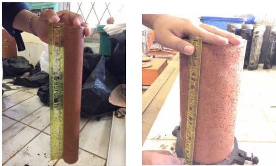
Fig. 4 DSM column samples (a) 3.75 and (b) 15 cm diameter
