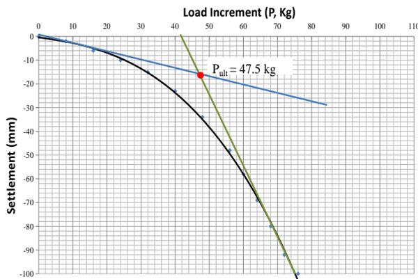
Fig. 8 Graph of load increment versus settlement
