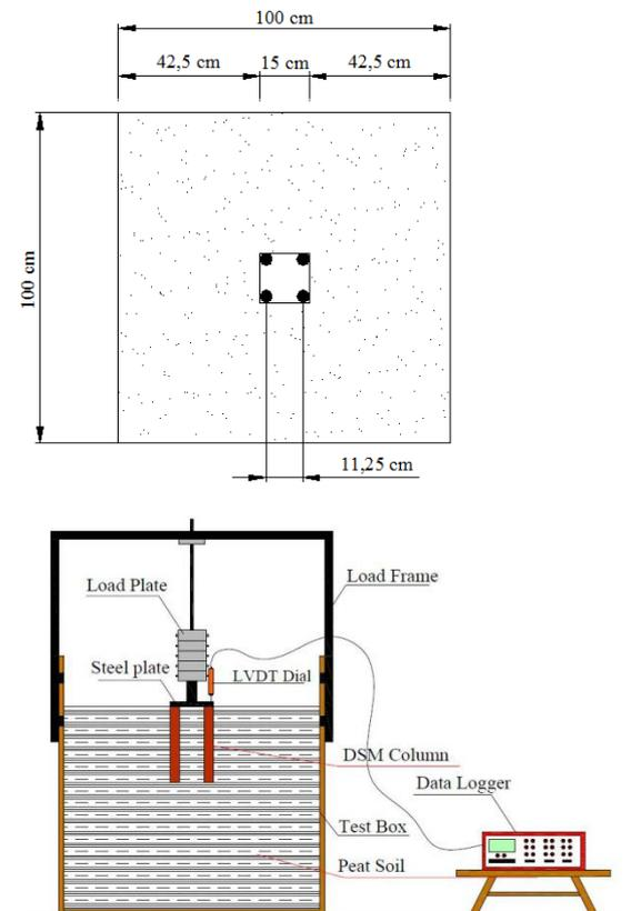
Fig. 6 DSM modeling scheme with 3.75 cm diameter with 4 columns
