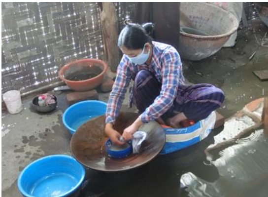
Fig. 4 Squeezing the gold-mercury amalgam
