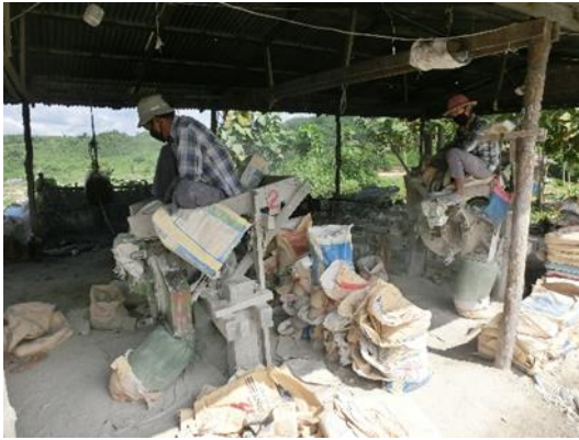
Fig. 3 A machine that powders gold ore
