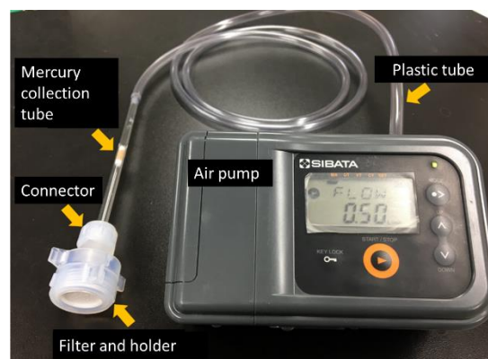
Fig. 7 Active sampler system operated with a dry battery
