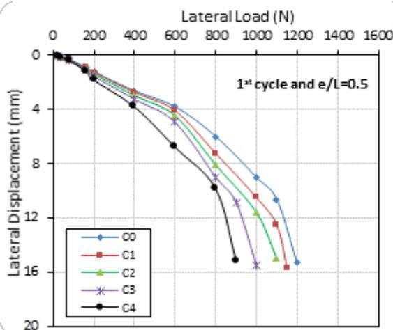
Fig.15 Total lateral displacement versus lateral load for  $e/L = 0.5$  at  $N = 1$  cycle
