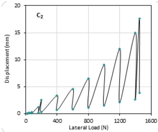
Fig.5 Displacement versus lateral load for soil sample C<sub>2</sub> and  $e/L = 0.25$
