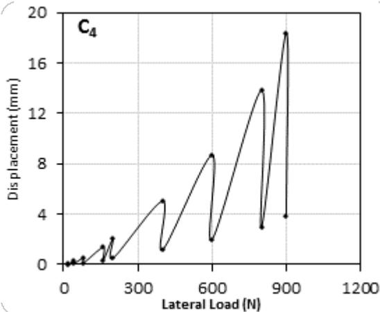
Fig.12 Displacement versus lateral load for soil sample C<sub>4</sub> and e/L = 0.5
