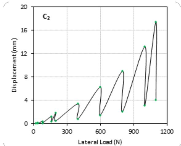
Fig.10 Displacement versus lateral load for soil sample C<sub>2</sub> and  $e/L = 0.5$
