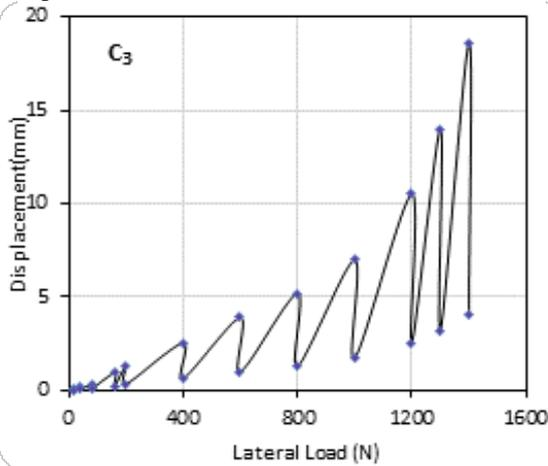
Fig.6 Displacement versus lateral load for soil sample C<sub>3</sub> and  $e/L = 0.25$
