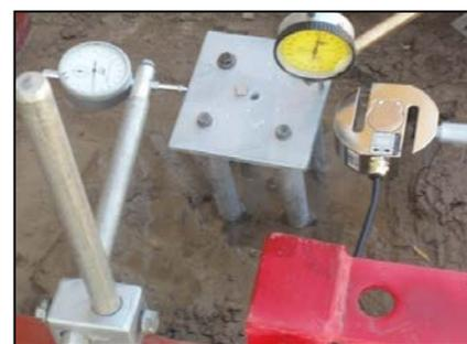
Fig.2 Instruments used in pile group testing
