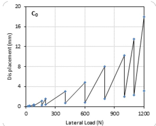
Fig.8 Displacement versus lateral load for soil sample C<sub>0</sub> and  $e/L = 0.5$
