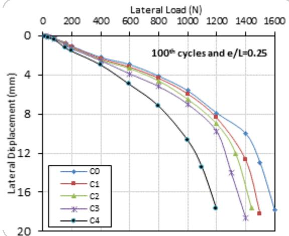
Fig.14 Total lateral displacement versus lateral load for e/L = 0.25 at N = 100 cycles
