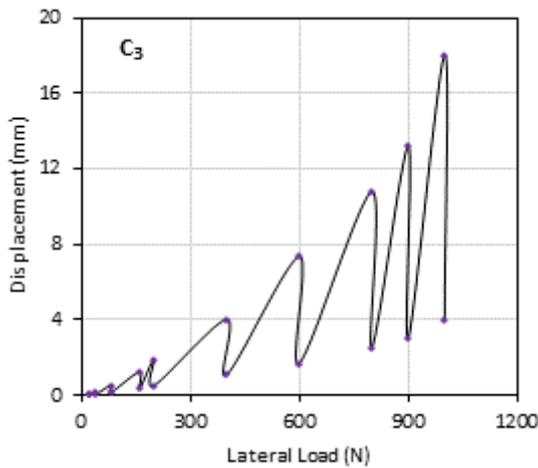
Fig.11 Displacement versus lateral load for soil sample C<sub>3</sub> and e/L = 0.5
