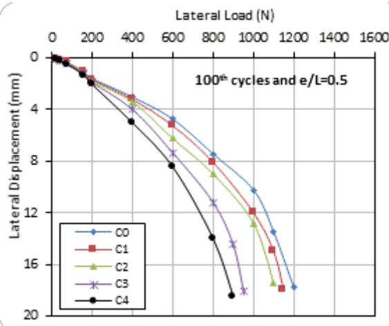
Fig.16 Total lateral displacement versus lateral load for  $e/L = 0.5$  at  $N = 100$  cycles
