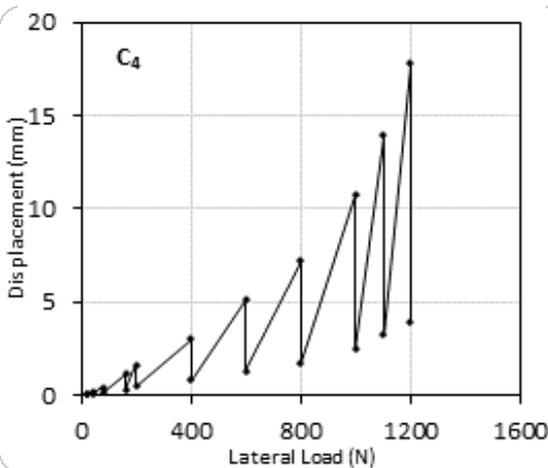
Fig.7 Displacement versus lateral load for soil sample C<sub>4</sub> and  $e/L = 0.25$
