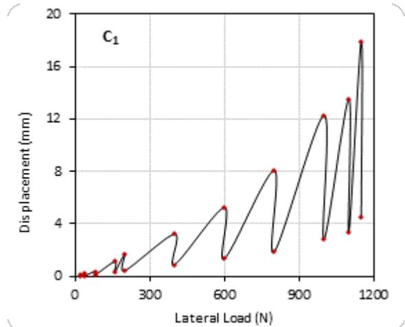
Fig.9 Displacement versus lateral load for soil sample C<sub>1</sub> and  $e/L = 0.5$
