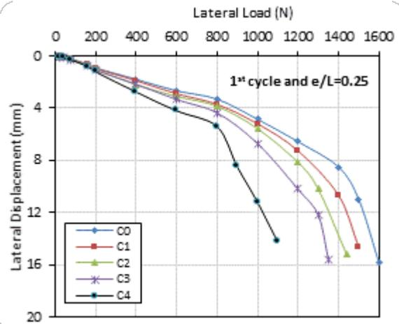
Fig.13 Total lateral displacement versus lateral load for e/L = 0.25 at N = 1 cycle
