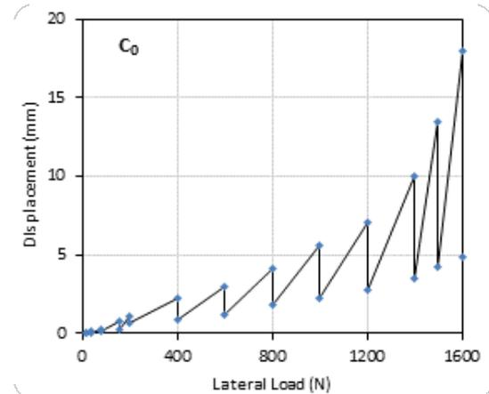
Fig.3 Displacement versus lateral load for soil sample C<sub>0</sub> and  $e/L = 0.25$
