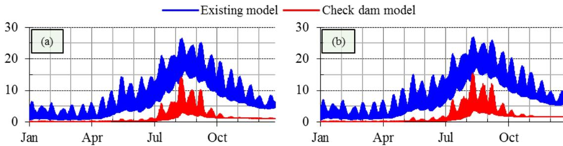
Fig.14 Salinity comparison between existing and check dam model at point 5 in (a) 2018 and (b) 2050. The vertical axis represents salinity in ppt
