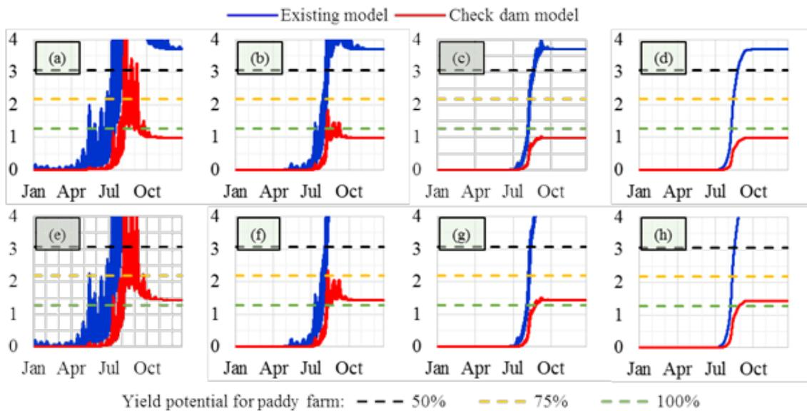
Fig.15 Salinity variations at points (a and e) 6, (b and f) 7, (c and g) 8 and (d and h) 9. Top row (a-e) for 2018 model and bottom row (e-h) for 2050 model. The vertical axis represents salinity in ppt
