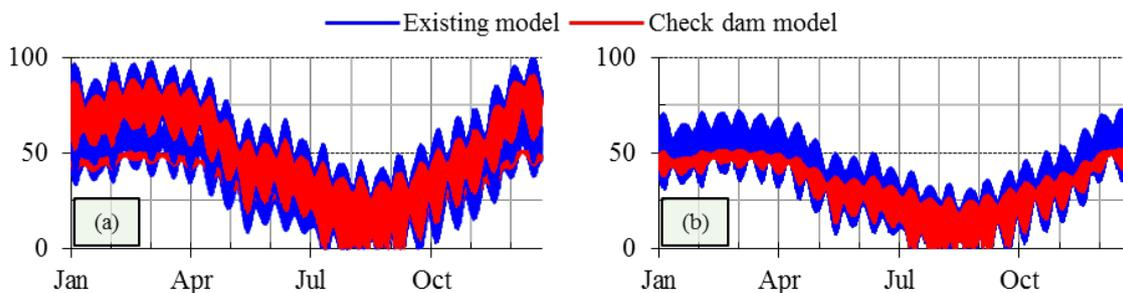
Fig.12 Current velocity comparison between existing and check dam model at point 5 in (a) 2018 and (b) 2050, the vertical axis represents velocity in cm/s
