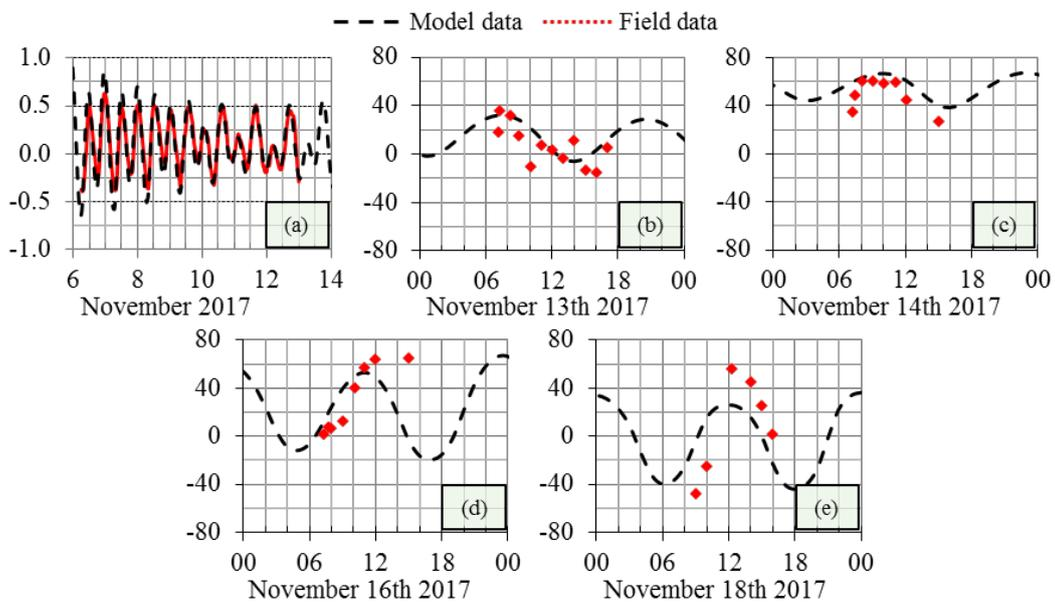
Fig.10 Result of (a) water level and (b-e) current velocity validation, vertical axes represent (a) water elevation in m and (b-e) current velocity in cm/s
