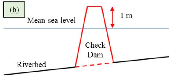
Fig.9 Check dam (a) locations and (b) concept design
