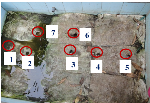
c. Lay out of observation of field CBR test for 7 points
