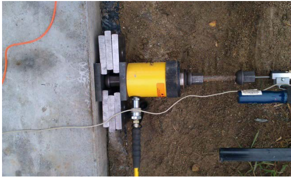
Fig. 2 The prestressing system
