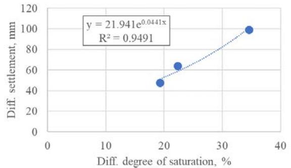
Fig. 22 The relationship between differential degree of saturation and differential settlement
