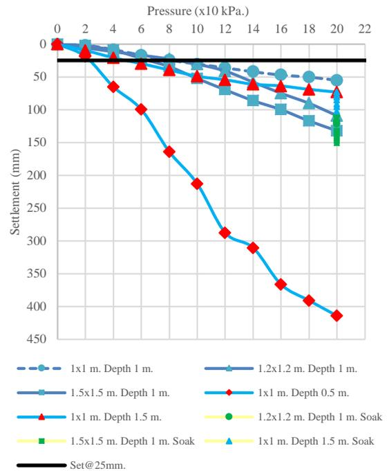
Fig. 19 Pressure-settlement curve; wet condition
