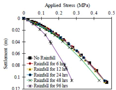
Fig.4 Footing 5x5 m. settlement and stress occurring with rainfall for soil type B [5]
