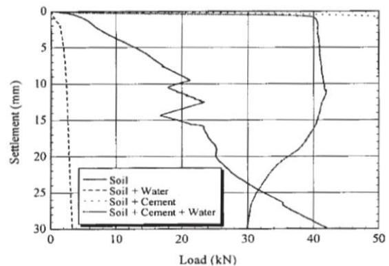
Fig. 6 The load – settlement curve of all test results [7]
