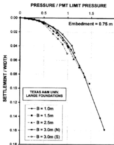
Fig.2 The pressure/PMT versus settlement/width curves [3]
