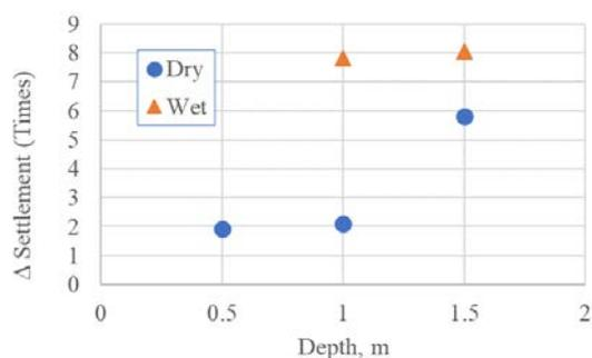
Fig. 24 The relationship between foundation depth and differential settlement after soaking
