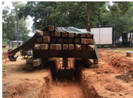
Fig. 10 Reaction beam and load pile transfer.
