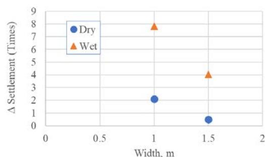
Fig. 25 The relationship between foundation width and differential settlement after soaking
