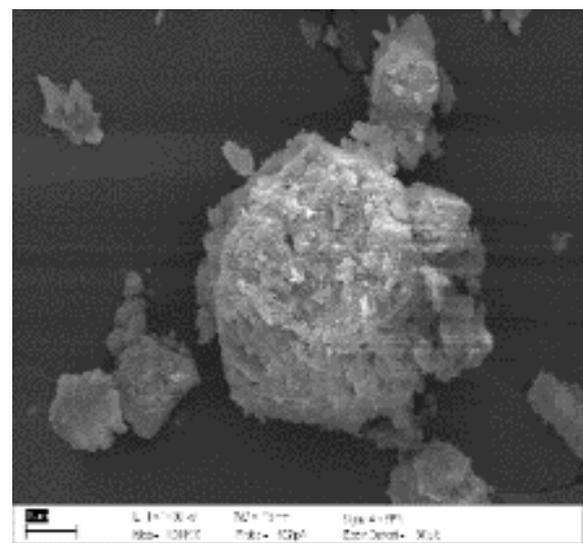
Fig. 14a Structure of Khon Kaen loess by SEM Test
