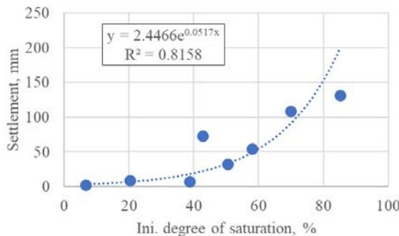
Fig. 21 The relationship between initial degree of saturation and settlement
