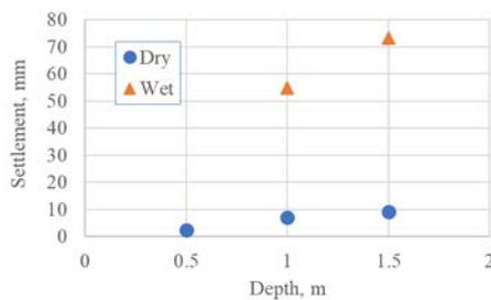
Fig. 18 The relationship between foundation depth and settlement
