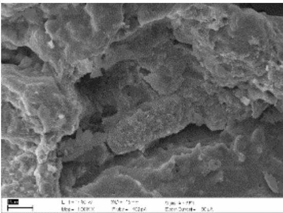
Fig. 14c Structure of Khon Kaen loess by SEM
