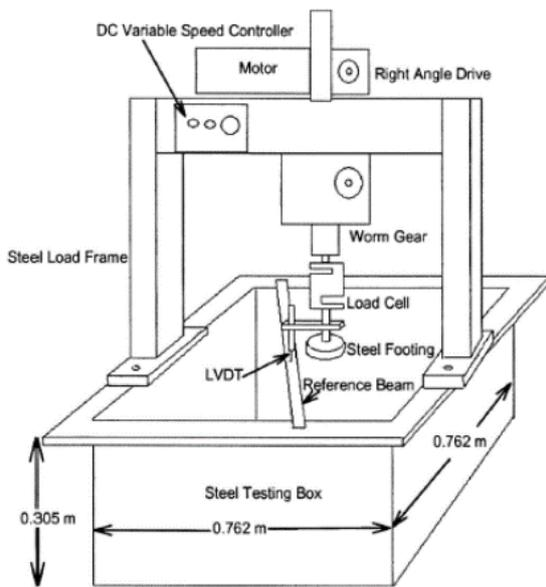
Fig. 7 Test equipment diagram, foundation size model used for testing [9]
