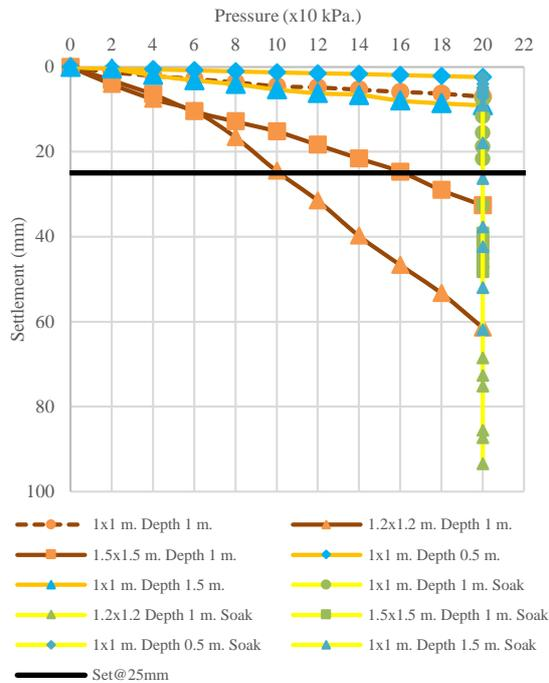
Fig. 17 Pressure-settlement curve; dry condition
