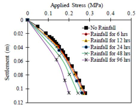
Fig.3 Footing 5x5 m. settlement and stress occurring with rainfall for soil type A [5]
