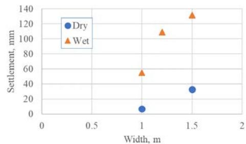
Fig. 20 The relationship between foundation width and settlement
