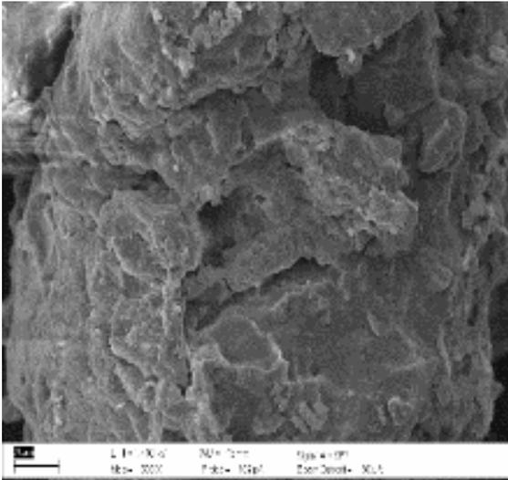
Fig. 14b Structure of Khon Kaen loess by SEM
