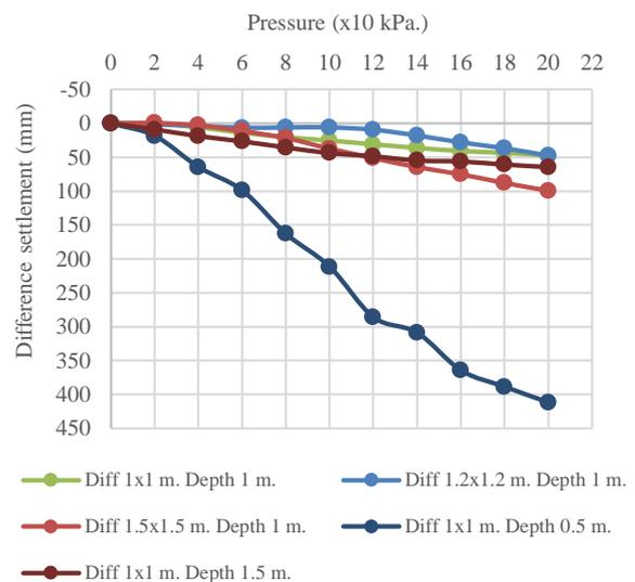
Fig. 23 Difference Settlement Foundation Testing
