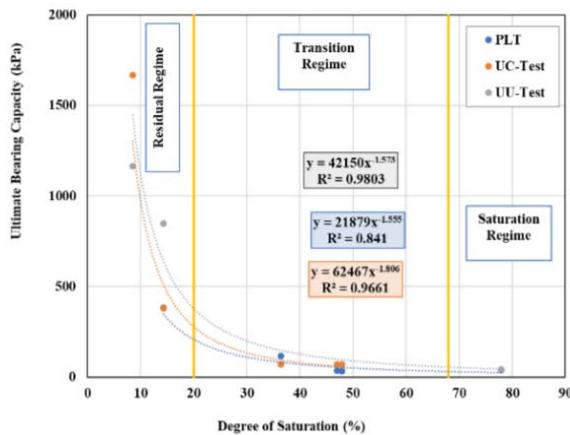
Fig. 5 The comparison of ultimate bearing capacity by Terzaghi's theory [6]
