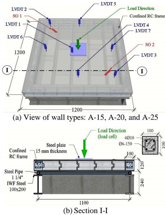
Fig. 2 Typical confined masonry walls
