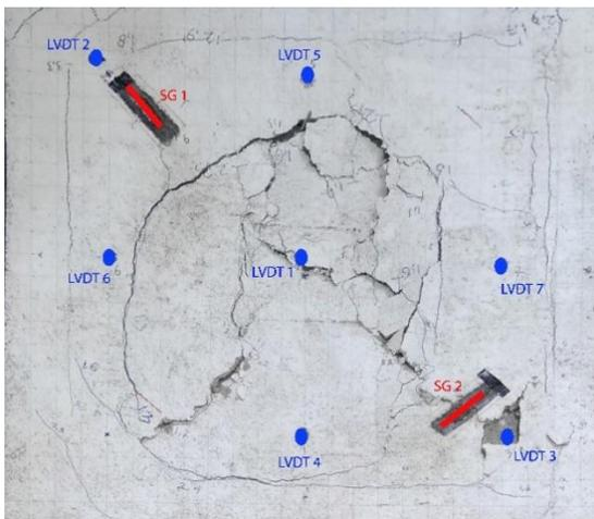
Fig. 6 Cracks propagation surrounding the point of load applied
