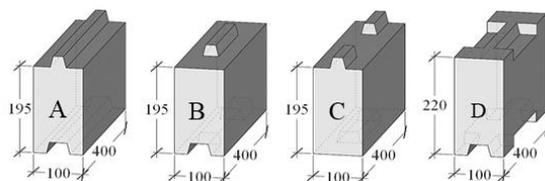
Fig. 1 Four models of interlocking concrete block
