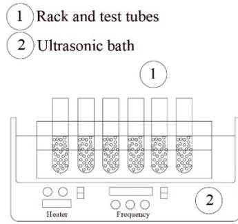
Fig. 1 Schematic diagram of the UAET.
