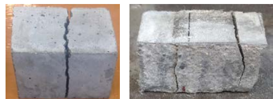
Fig. 9 An example shape of prismatic specimens remained after compressive loading at (A) plain geopolymer mortar (AAM-VI) and (B) geopolymer fiber reinforced composite (AAM-F).
