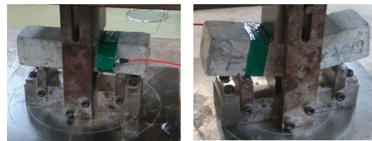
Fig 1. Flexural test on mortar reinforced fiber composite (A) before and (B) after failure
