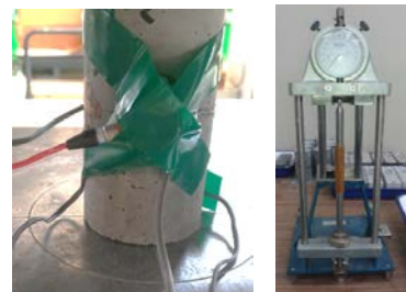
Fig 2. Compressive test and drying shrinkage test on mortar reinforced fiber composite specimens
