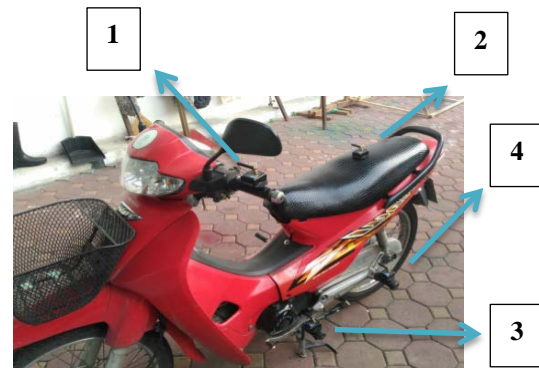
Fig. 3 Experimental allocation of accelerometers over the specimen motorcycle; (1) left hand, (2) seat, (3) left front footrest, and (4) left rear footrest.
