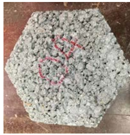
Fig.3 Porous paver concrete block in a hexagon shape
