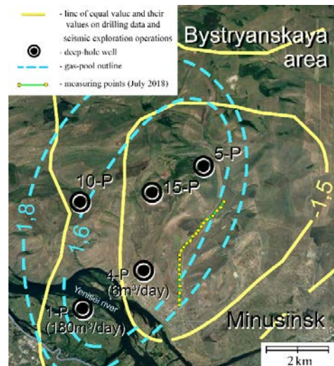
Fig. 4. Observations using conventional seismic survey and passive seismoelectric method.
