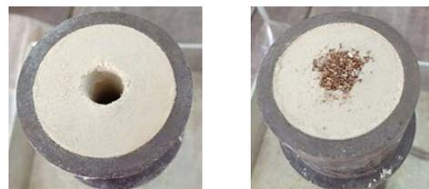
Fig.3 (a) Before installation of CCS column into the kaolin clay. (b) After installation of CCS column into the kaolin clay
