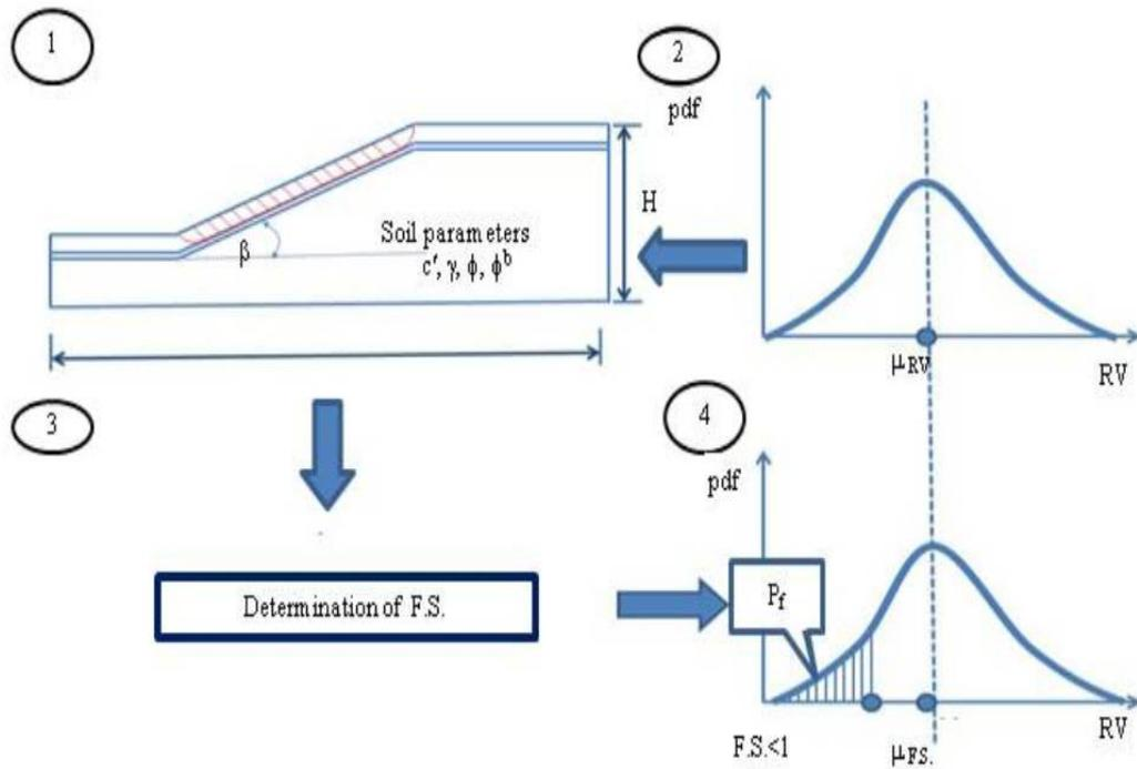
Fig. 2 Probabilistic slope stability analysis process (Adapted from [6])
