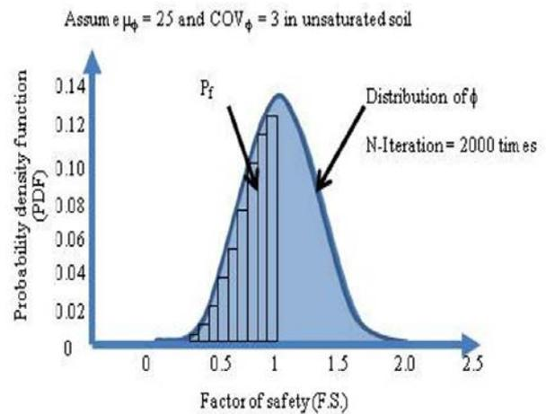
Fig. 4 Assessment of the system probability of failure
