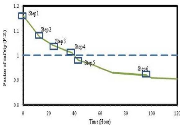
Fig. 3 Time-step versus factor of safety during the rainfall
