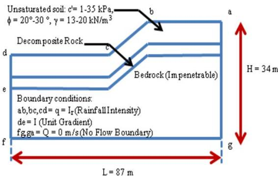
Fig. 1 Slope geometry and boundary conditions for unsaturated soil slope
