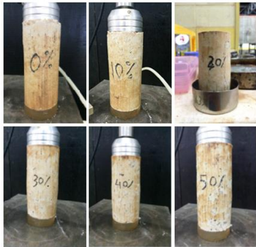
Fig. 11 Failure modes samples in UCS tests
