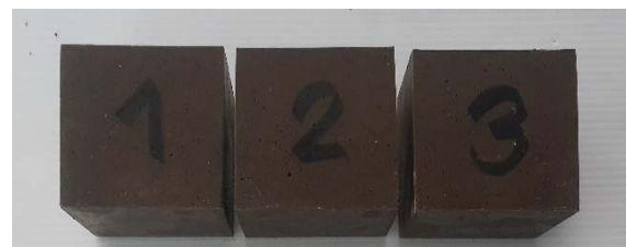
Fig.3 The sample of fluidized bed coal-bark fly ash geopolymer mortar containing additives
