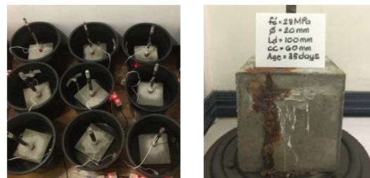
Fig. 1 Concrete cubes under accelerated corrosion
