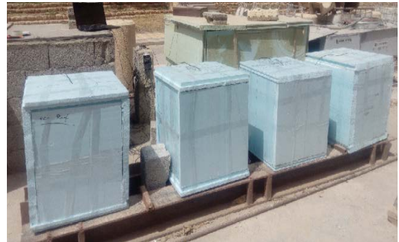
Fig. 2. Two constructed chambers with a set of four polystyrene boxes.
