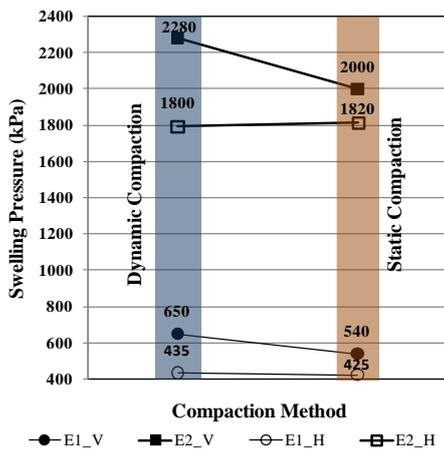
Fig. 6. Swelling Pressure versus Compaction Method
