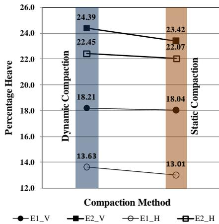
Fig. 5. Percentage Heave versus Compaction Method
