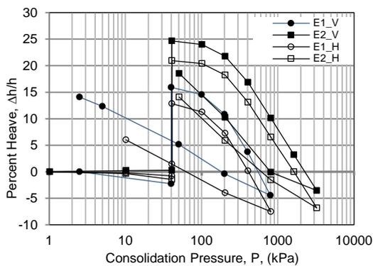
Fig. 7. Percent Heave versus Consolidation Pressure for Dynamic Compaction
