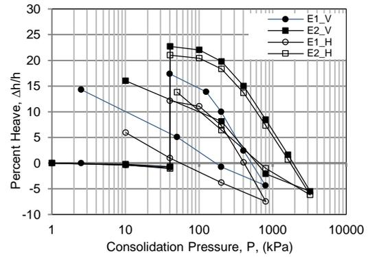
Fig. 8. Percent Heave versus Consolidation Pressure for Static Compaction
