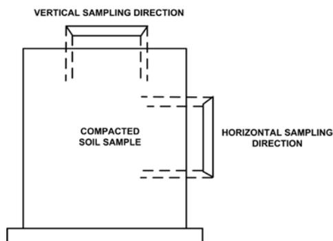
Fig. 4. Schematic diagram of horizontal and vertical sampling
